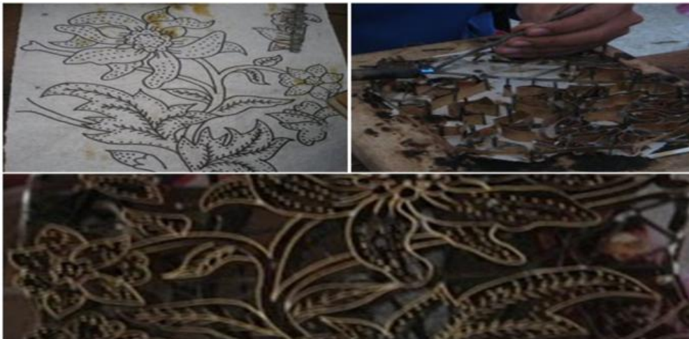
Figure 3. Block making process [11].
