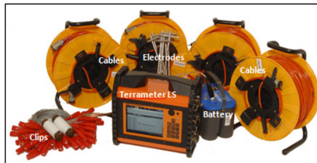
Figure 3. Equipment used for ERI
