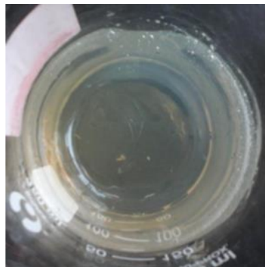
Figure 5. Photo showing solidification occurred from the outer surface inwards.
