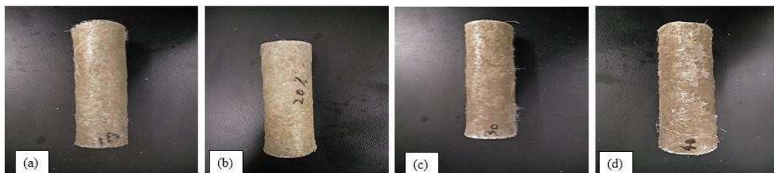
Figure 2: Pipe samples by different ratio of fiberglass reinforced plastic waste (FRPW); (a) 1:0.5, (b) 1:1.0, (c) 1:1.5, (d) 1:2.0
