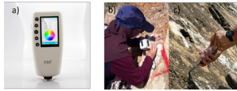
Figure 3. Insitu testing; a) Colorimeter testing device, b) methods to setting up the colorimeter, c) validation results using L-type Schmidt hammer.
