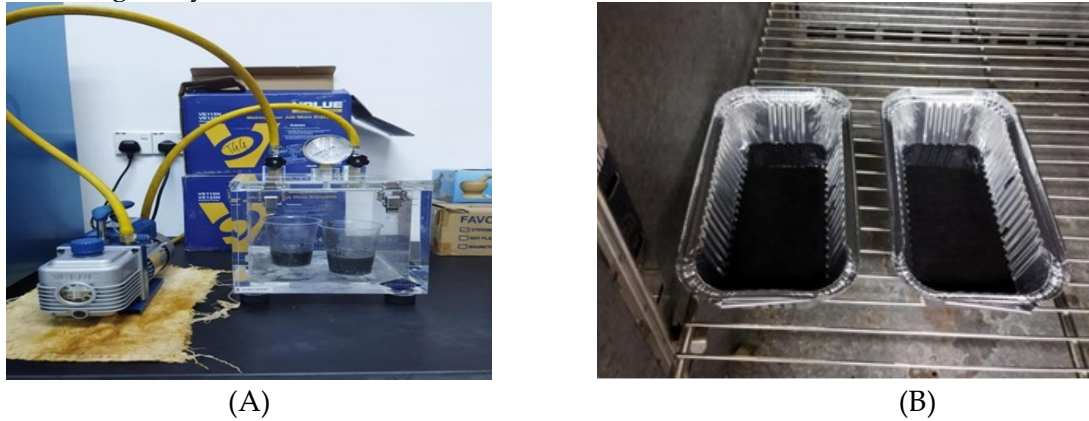
Figure 1. Experimental Setup and Process. (A) Sample Mixture in Vacuum Chamber, (B) Curing Process in the Oven.
