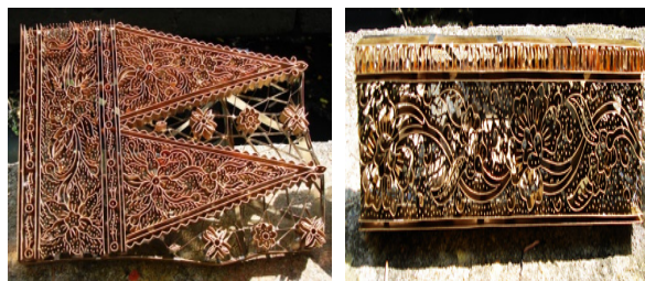
Figure 1 and 2. Batik copper block, which is Malaysian Tradition method of making batik sarong
