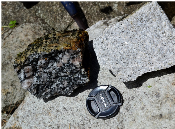
Figure 3. The coarse grained granite dominated with hornblend (left) and the coarse grained granite dominated with quartz and feldspar.
