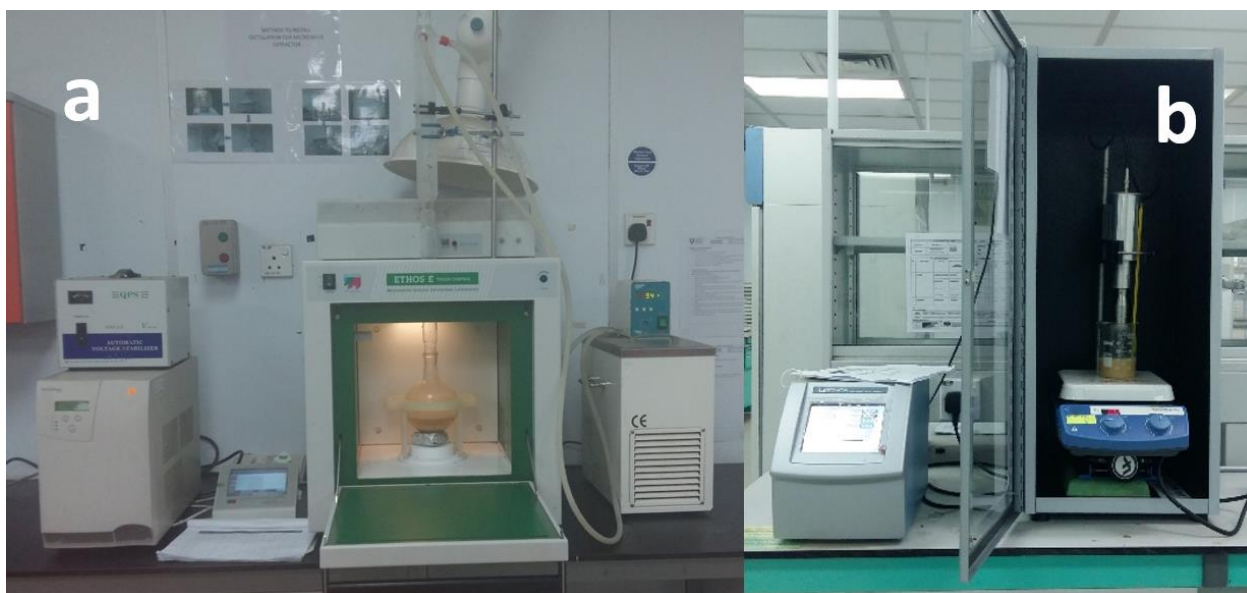
Figure 1. The extraction instruments (a) Microwave apparatus (b) Ultrasound processor with the attached hot plate.
