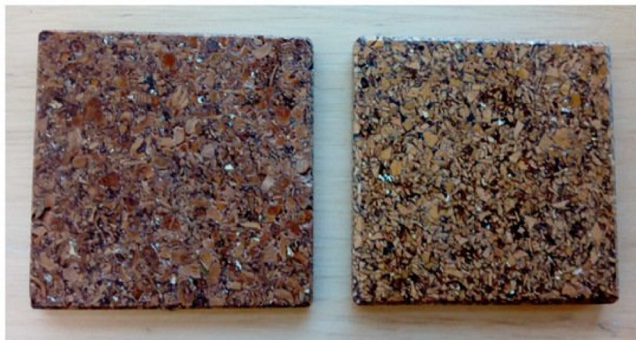
Fig. 11 – Hazelnut (left) and walnut shell (right) particleboard (Barbu et al. [50], open access).
