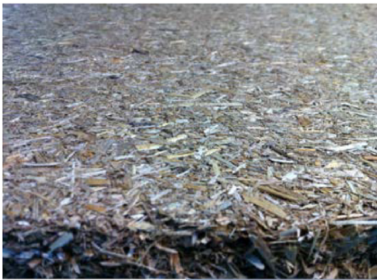
Fig. 12 – Reed canary grass particleboard by Trischler et al. [139], licensed under Creative Commons Attribution-NonCommercial 4.0 International License.
