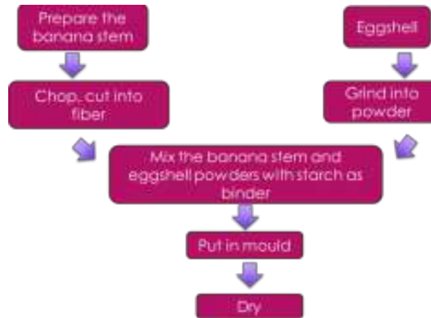
Figure 1. The overview of BioG Pot preparation.
