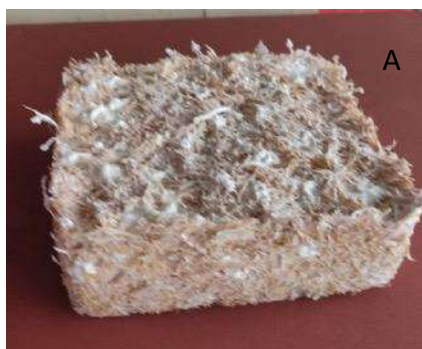
Figure 1: MUSM cardboard/flat board prototype. Figure 1A shows the mycelium has covered the mold shape; 1B shows that cardboard/flat board from MUSM.
