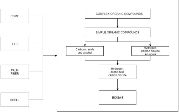
Fig. 4. Degradation steps of the anaerobic digestion process [28]
