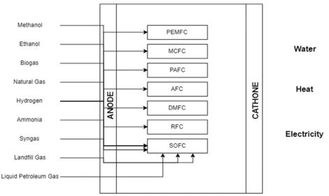
Fig. 1. Concept of a fuel cell system
