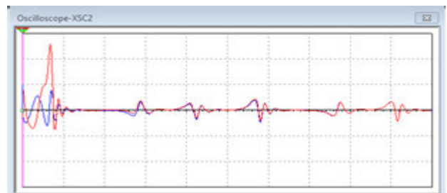
FIGURE 26. Time evolution of master system first state x_1 (red color) and slave system first state y_1 (blue color).
