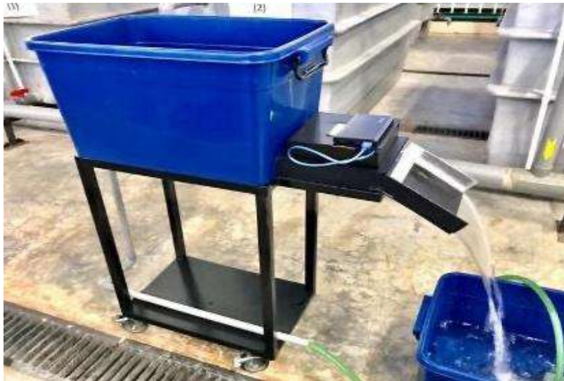
Figure 1: Fish fry Mobile Auto Counter (FryMAC)
