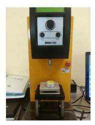
Figure 3: The hardness of lip balm was analysed using Ametek Brookfield CT-3 Texture Analyzer
