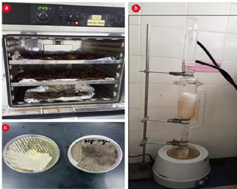
Fig. 4 – a) Oven dry of AV leaves, b) Soxhlet extraction method, c) Candida albicans and Aspergillus niger SDA method [87].
