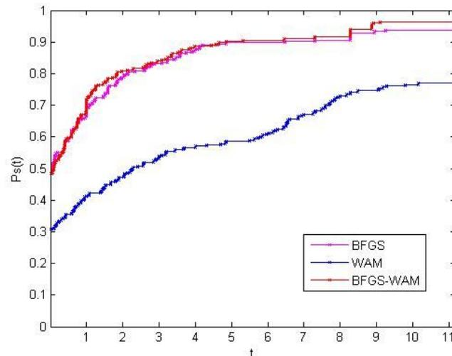
**Figure 2** Performance profile of BFGS, WAM and BFGS-WAM methods based on CPU time
