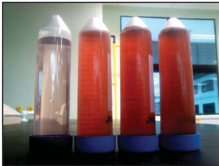
FIGURE 5. The treated dye effluent (modified pH from left: pH 3, 5, 7 and 9) with AC60.
