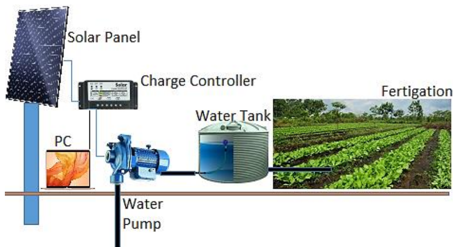
Figure 1. The concept of solar system with IoT-based technology to power water pump for the fertigation
