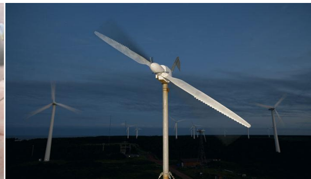
Figure 5. Wind Turbine blades inspired by Whalefin. Source: https://materialdistrict.com/article/humpback-whales-inspire-next-generation-wind-turbine-technology/humpback-whales-inspire-next-generation-wind-turbine-technology-1/
