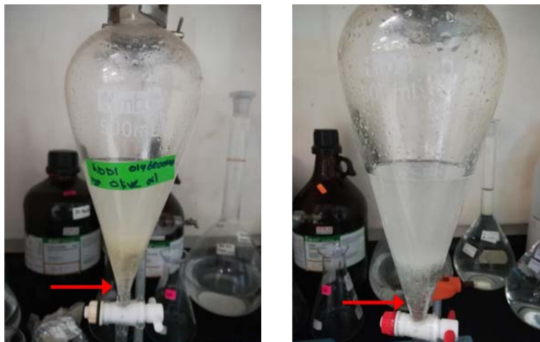
Figure 2. Broth cultures mixed with olive oil (left) and motorcycles oil (right) for lipid extraction using chloroform and methanol as solvent. Red arrow shows the chloroform layer.
