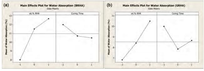
Fig. 6. (a) Main Effects Plots for Water Absorption (BRHA). (b) Main Effects Plots for Water Absorption (GRHA).
