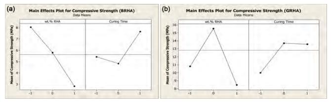
Fig. 4. (a) Main Effects Plots for Compressive Strength (BRHA). (b) Main Effects Plots for Compressive Strength (GRHA).
